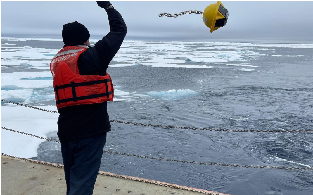
Figure 1: CWO2 Latin deploys a Sofar spotter from the deck of USCGC Healy.
